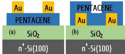
**Figure 1. a) Top contact transistor b) Bottom contact transistor based on pentacene as a semiconducting layer.[21]**
