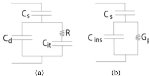
**Figure 6. (a) Interface model of the capacitor (b) Model of the capacitor at accumulation mode [12].**
