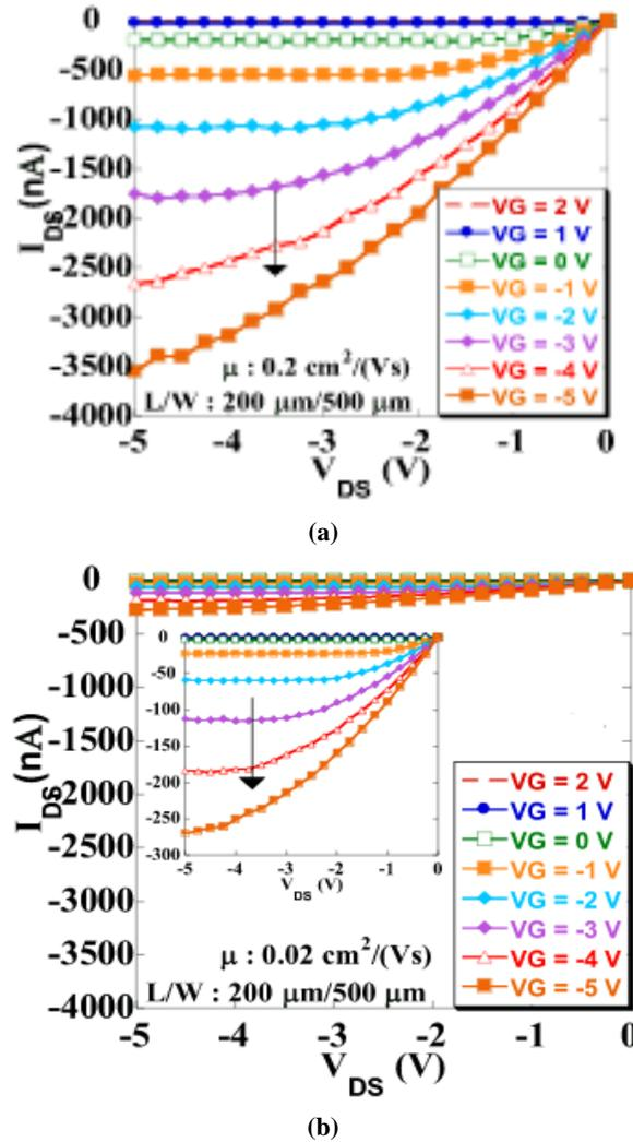
**Figure 2.**  $I_D$ - $V_D$  characteristics of different structures of pentacene OFET (a) Top Contact (b) Bottom Contact [21].
