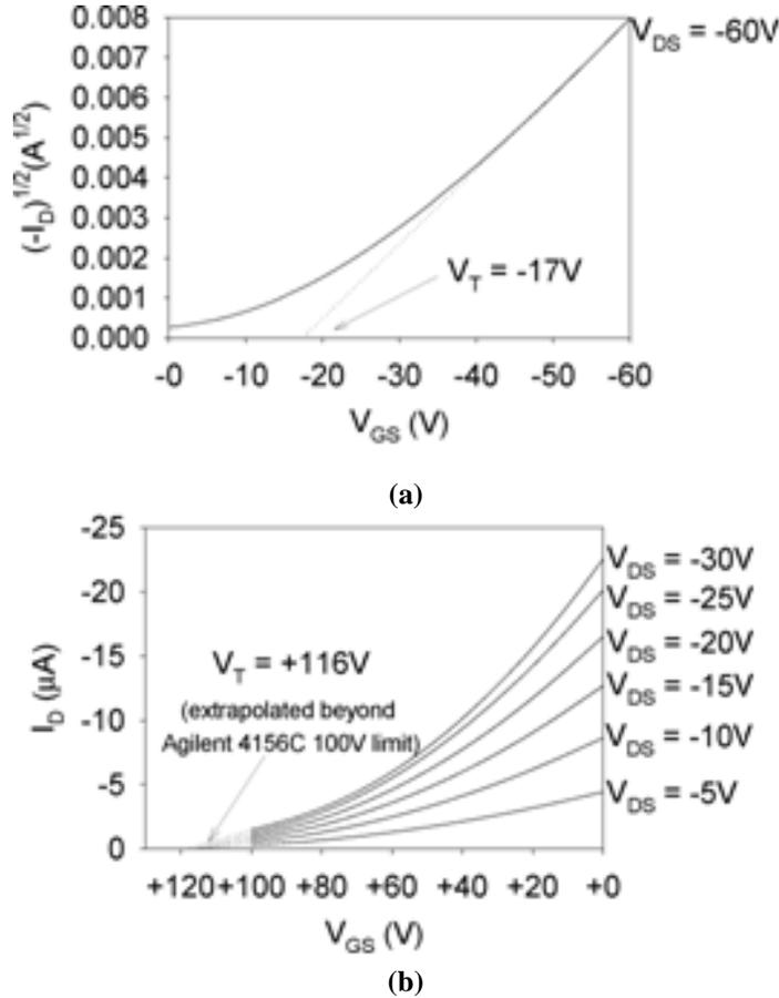
**Figure 4. Threshold Voltage of OFET Devices (a) Devices 1 (b) Devices 2 [12].**
