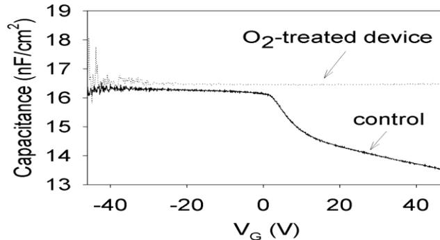
**Figure 5. C-V curve of device 1 shows all accumulation, flat band, and depletion mode which device2 does not, only accumulation region [12].**
